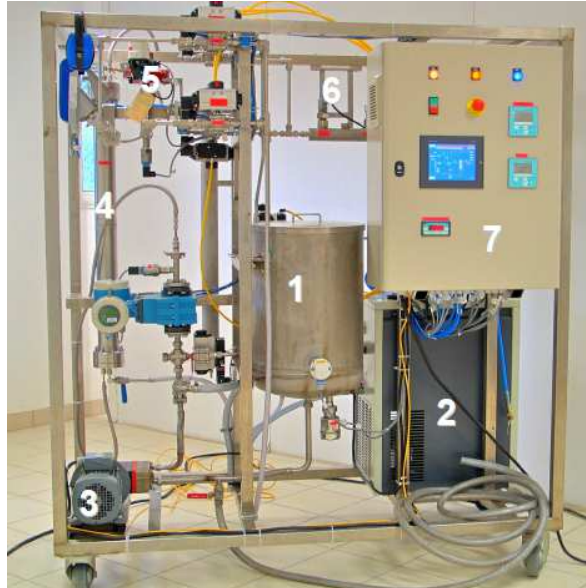
Figure 2. Presentation of the nanofiltration pilot used in this study: (1) feed tank; (2) temperature control loop; (3) pressure pump; (4) 2.5” stainless steel pressure vessel; (5) pressure regulating valve; (6) sampling loop; (7) programmable logic controller.
